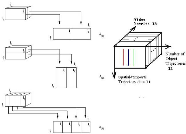
**Fig. 1.** Flattening a  $3^{rd}$  order motion event tensor for multiple trajectories representation.
