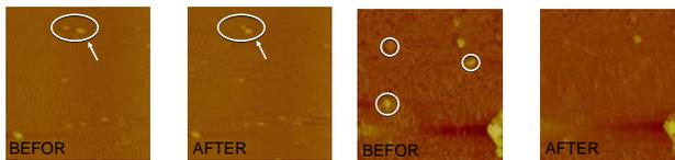
Figure 8. Nanomanipulation using Atomic Force microscope to individually move particles on the surface.
