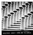
Figure 2. Photoresist pillars fabricated at the University of New Mexico
