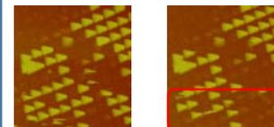
Figure 10. Nanomanipulation using Atomic Force microscope in liquid environment (Acetone)
