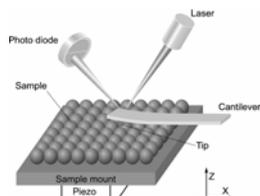
Figure 3. Schematic of Atomic Force Microscope operation
