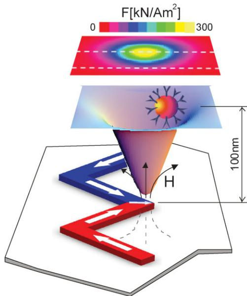
**Figure 1.** Bottom: sketch of a Py nanostrip with a DW in a corner and of the corresponding potential energy surface for a magnetic bead carrying antibodies on a plane at 100 nm from the Py structure. Top: color intensity plot of the modulus of the attractive force per unit magnetic moment.
