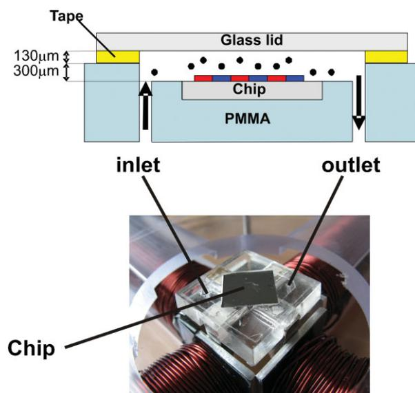
**Figure 5.** Top: Sketch of the microfluidic cell, where inlet and outlet are connected to syringe pumps. Bottom: The microfluidic cell inserted in the middle of the magnetic poles is slightly elevated with respect to the maximum field plane in order to exploit the field gradient to attract the particles on the chip surface.
