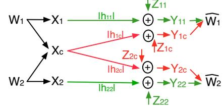
Fig. 3. The transformed channel for Th. 4.
