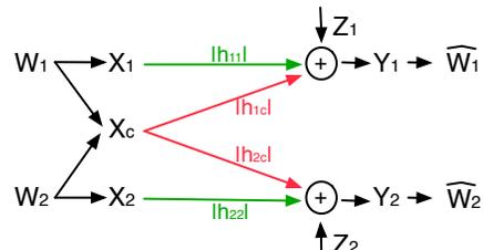
Fig. 1. The GPC-CR channel with two messages  $W_1$  and  $W_2$  known non-causally at the Cognitive Relay (CR) with subscript  $C$ .
