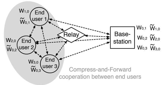
Fig. 1. Our physical channel model consists of multiple independent bi-directional desired communication flows (indicated by arrows) between multiple terminal nodes, a single relay node, and a single base-station.  $W_{i,j}$  denotes the message from node  $i$  to node  $j$ , while  $\tilde{W}_{i,j}$  is the estimate at node  $j$  of the message  $W_{i,j}$ .
