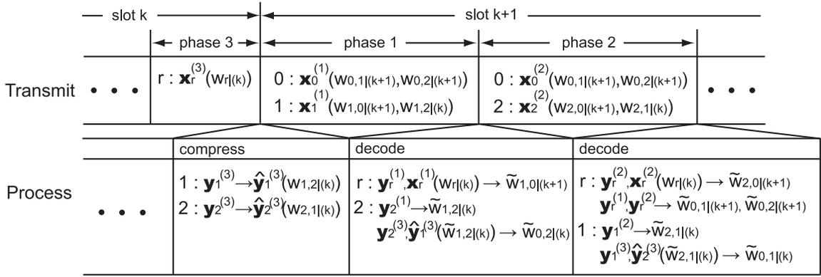
Fig. 2. An example of the PMABC protocol with terminal-node cooperation with two end-users  $m = 2$  and one base-station.
