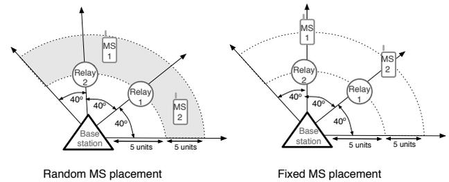
Fig. 6. Simulation setup: Relays are at equal distance from the base station and are spaced at angles  $40^\circ$  on an arc of radius 5 units. Two different models for mobile placement are simulated: MS positions are random in the shaded sector for the *random MS* placement, or at the fixed points in the *fixed MS* placement.
