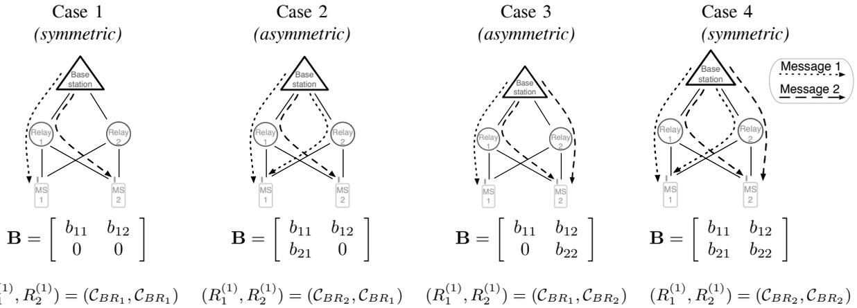
Fig. 4. Four dual-message knowledge scenarios when  $|h_{BR_1}| \geq |h_{BR_2}|$ , and the corresponding linear precoding matrices  $\mathbf{B}$ .
