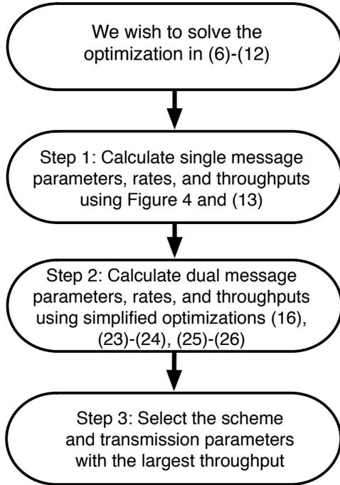
Fig. 5. Flowgraph of the maximum throughput optimization which could lead to asymmetric relay cooperation.
