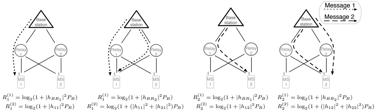
Fig. 3. Four message knowledge scenarios when  $|h_{BR_1}| \geq |h_{BR_2}|$ , and a single message is sent. The corresponding phase 1 and phase 2 rates are illustrated.
