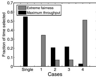
Fig. 7. Percentage of time the single message case and the 4 dual-message cases are chosen under *random MS* placement.  $P_R = P_B = 1000$ , radius=10 units.
