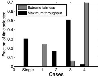
Fig. 10. Percentage of time the single message case and the 4 dual-message cases are chosen under *fixed MS* placement.  $P_R = P_B = 1000$ , radius=10 units.
