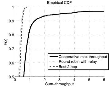
Fig. 11. CDF of sum throughput under the max throughput criterion, *fixed MS* placement.
