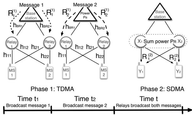
Fig. 2. Transmission takes place in two phases: in phase 1 the BS broadcasts messages in TDMA fashion: message 1 for  $t_1$  time units, then message 2 for  $t_2$  time units. During phase 2 the relays simultaneously transmit all received messages to the MSs. Illustrated are the channel gains, power constraints, rates, and input-output variables.
