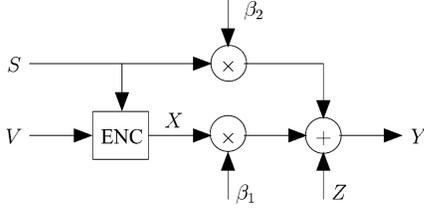
Fig. 4. Communications over a fading channel with a fading interferer whose signal, but not fading coefficient, is known at the transmitter.
