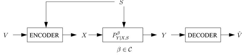
Fig. 1. Memoryless compound channel with side information at the transmitter.
