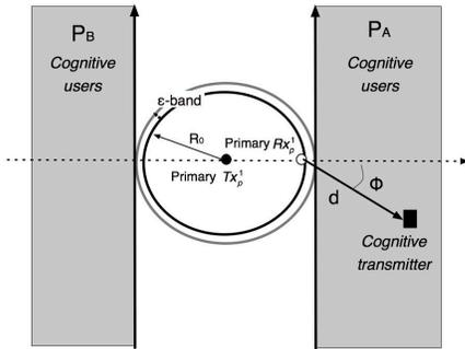
Fig. 4. Another lower bound on the expected interference at the primary receiver is obtained by approximating the interference region by two half-planes  $P_A$  and  $P_B$ . The region between these planes is free from cognitive transmitters.
