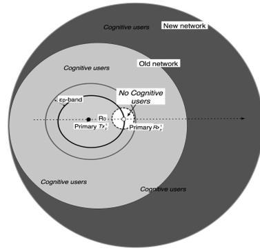
Fig. 5. An upper bound on the expected interference at the primary receiver is obtained by forming a cognitive-free circle of radius  $\epsilon_p$  around the primary receiver and enlarging the network radius, centered at the primary receiver, to  $R + R_0$ . All cognitive transmitters now lie within these new boundaries.
