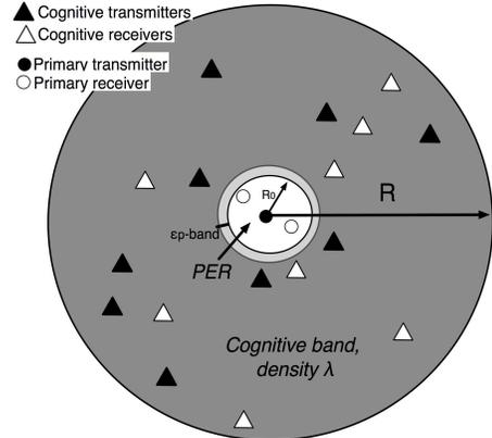
Fig. 1. A cognitive network consists of a single primary transmitter at the center of a *primary exclusive region* (PER) with radius  $R_0$ , which contains its intended receiver. Surrounding the PER is a protected band of width  $\epsilon_p > 0$ . Outside the PER and the protected bands,  $n$  cognitive transmitters are distributed randomly and uniformly with density  $\lambda$ .
