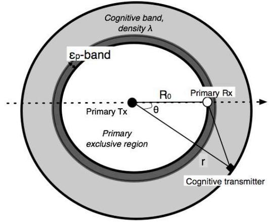
Fig. 2. Worst-case interference to a primary receiver: the receiver is on the boundary of the primary exclusive region of radius  $R_0$ . We seek to find  $R_0$  to satisfy the outage constraint on the primary user.
