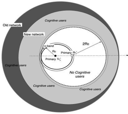
Fig. 3. A lower bound on the expected interference at the primary receiver is obtained by forming a cognitive-free circle of radius  $2R_0$  around the primary receiver and reducing the network radius, now centered at the primary receiver, to  $R - R_0$ . All cognitive transmitters now lie within these two new boundaries.
