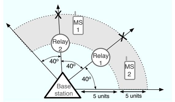
Fig. 3. Geometric distribution: relays at equal distance, spaced at angles  $40^\circ$  on arc of radius 5 units, mobiles random in shaded sector for the random MS placement, or at the points marked X for the fixed MS placement.
