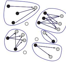
Fig. 1. A wireless network consisting of cognitive and/or non-cognitive devices. Black nodes are senders ( $S_i$ ), striped nodes are receivers ( $R_i$ ), and white nodes are inactive. A directed edge is placed between each desired sender-receiver pair at each point/period in time. Here the active links have been decomposed into subsets ( $S_i, R_i$ ) of *generalized MIMO channels*.
