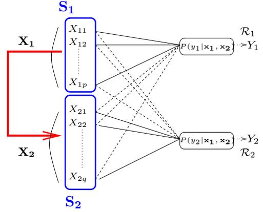
Fig. 2. The genie-aided inter-cluster cognitive radio MAC channel with inputs  $\mathbf{X}_1 := (X_{11}, \dots, X_{1p})$ ,  $\mathbf{X}_2 := (X_{21}, X_{22}, \dots, X_{2q})$ , and outputs  $Y_1$  and  $Y_2$ .
