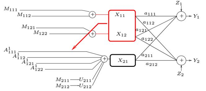
Fig. 6. The modified Gaussian genie-aided cognitive radio multiple access channel for  $p = 2, q = 1$ , with inputs  $X_{11}, X_{12}, X_{21}$ , auxiliary random variables  $M_{111}, M_{112}, M_{121}, M_{122}, M_{211}, M_{212}, U_{211}$  and  $U_{212}$ , outputs  $Y_1$  and  $Y_2$ , additive Gaussian noise  $Z_1$  and  $Z_2$  and interference coefficients.
