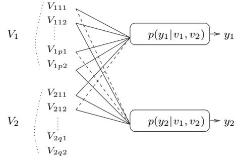
Fig. 4. The equivalent channel with random variables  $V_{1ik}$  and  $V_{2jk}$ . These are two overlapping, and interfering MAC channels. The solid lines are desirable connections while the dashed lines are interference.
