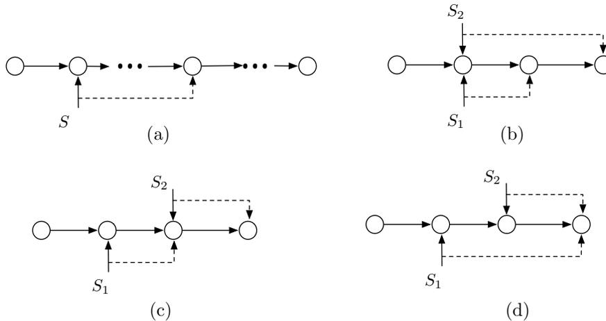
Fig. 3. Extensions to multi-relay and multi-interference channels with channel state known at the receiver.
