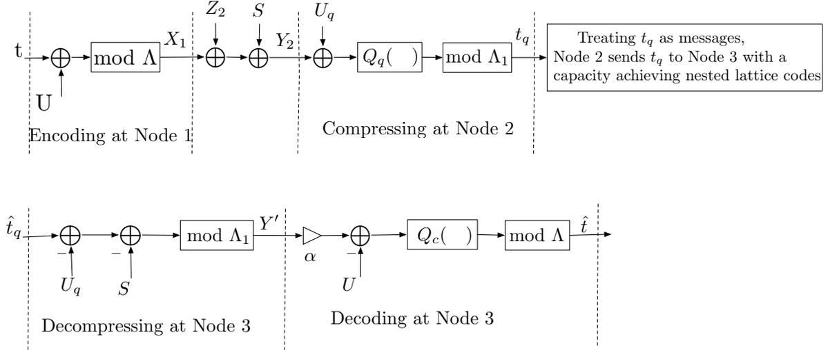
Fig. 2. Nested-lattice encoding and decoding scheme of Theorem 1.
