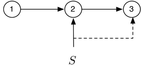
Fig. 1. Canceling known interference in a two-hop network. Solid lines indicate interference, dotted lines indicate its non-causal knowledge.
