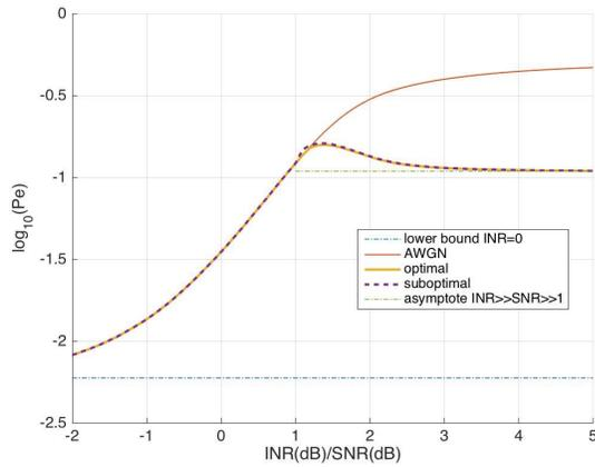
Fig. 2. BER for BPSK with  $S = 5$  dB vs.  $l$  in dB.
