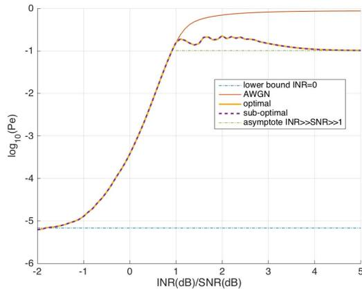
Fig. 4. BER for 8-PAM with  $S = 10$  dB vs.  $I$  in dB.
