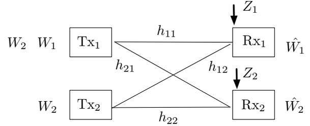
Fig. 1. The ergodic fading Gaussian cognitive interference channel.
