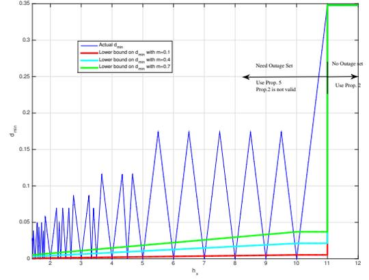
Fig. 2: Minimum distance (blue line) for the sum-set  $h_x X + h_y Y$  as a function of  $h_x$  for fixed  $h_y = 1$  and for  $X \sim Y \sim \text{PAM}(10, 1)$ .
