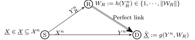
Fig. 3: An  $n$ -shot protocol  $(n, \underline{\mathcal{X}}, h, g)$  for zero-error communication over a PRC  $(\mathcal{X}, p(y, y_R|x), \mathcal{Y} \times \mathcal{Y}_R)$ , with a codebook  $\underline{\mathcal{X}}$ , a relaying function  $h$  and a decoding function  $g$ .
