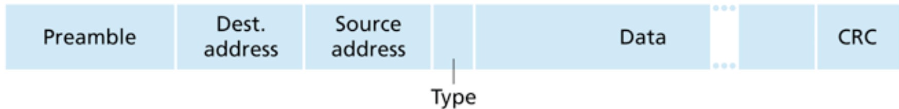
Figure 5.22 ♦ Ethernet frame structure
