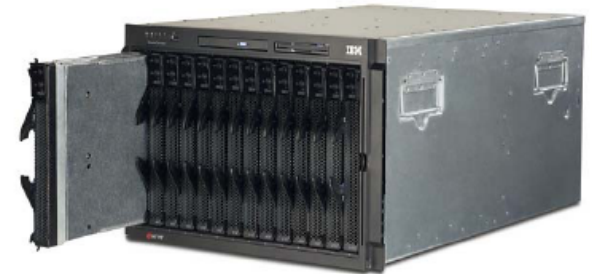
7U rack with 14 IBM LS21 Blades
